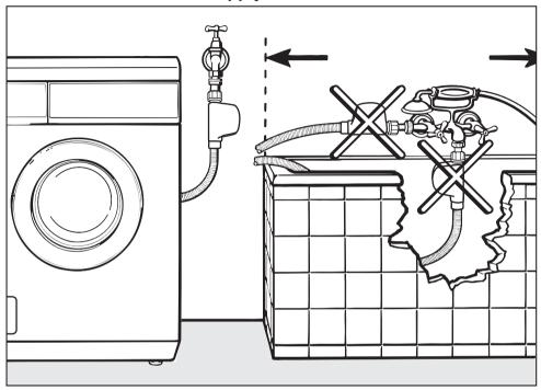
The plastic casing of the safety valve contains electrical components. The Water-proof system must only be connected to its own stopcock. It must not be connected to mixer taps or similar and must not be fitted in areas where there is the risk of water or other liquids reaching it.
